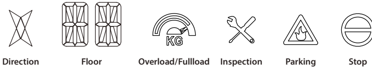
Figure 1-12 MT70-HCB-U1 state display description
